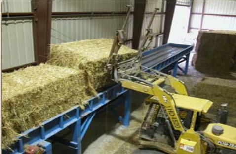
Switchgrass bales being loaded onto the conveyor which then goes
