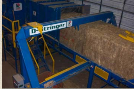
through the de-stringer to remove the bale strings...
