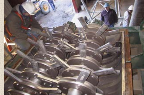
...then transported by conveyor to the "Eliminator" which grinds the switchgrass.
