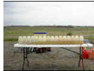
Run-off is collected for a duration of 15 minute at five minute intervals during each hour and twenty rainfall simulation.
