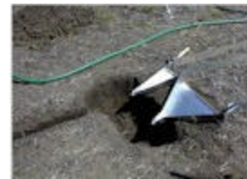
Run-off collection site before rainfall simulation begins.
