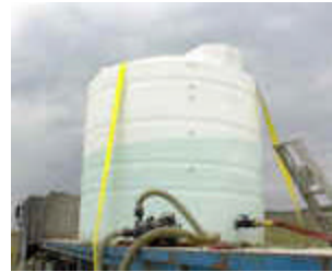
A 3,000 gallon water tank is on-site to supply water for rainfall simulator.
