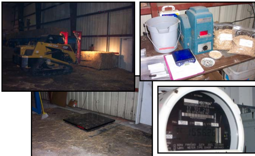
Weighing bale (top left) on digital scale (bottom left). Infrared moisture balance, scales, and sampling supplies (top right). Electric meter at "Biosilo" (bottom right).
