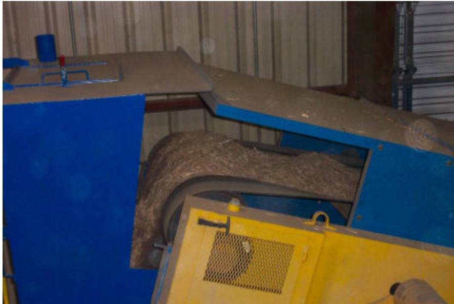
Debaled switchgrass flowing off of Take-away Conveyor into "Eliminator" infeed.
