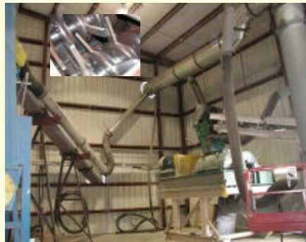
Attrition Hammermill and Pneumatic Conveyor
