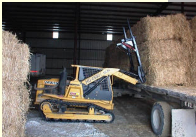
Telescopic forklift with hydraulic push off bars for handling biomass
