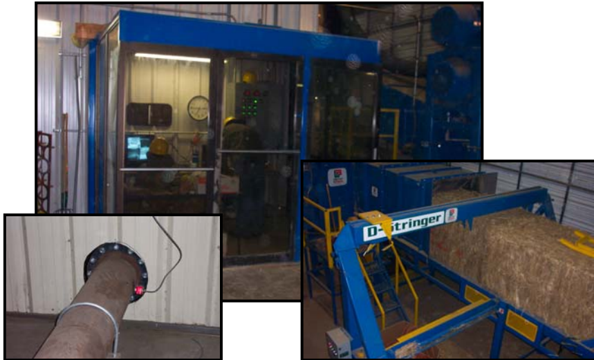
D-Stringer (bottom right) counts bales and displays running total on operator panel in "Biosilo" control room (bottom right). Ultrasonic ON/OFF sensor on biomass supply pipe (bottom left).
