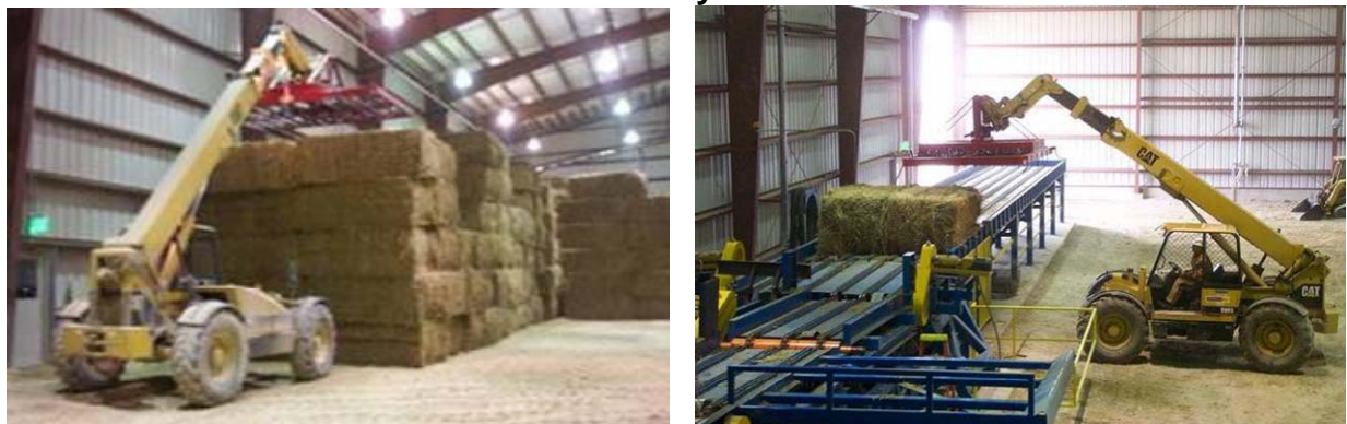
Exhibit 25 Twin Bale Conveyor and Teleboom Loader
