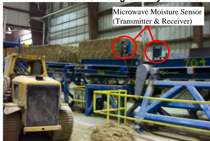
Exhibit 27 Bale Sensing Conveyor Photo
